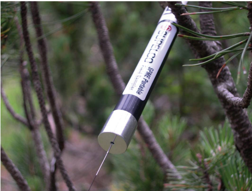
Figure 2. Portable SPME employed to sampling the VOCs in the park.
