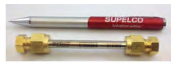
These passive sampling tubes work by collecting the air sample without the need of an air sampling pump to physically pull the air sample through the adsorbent. The FLM Carbopack X tube relies on the natural movement (of the HAP's) across a concentration gradient inside the inlet of the tube called the "air gap". The volatile HAPs travel through the air gap and are adsorbed by the Carbopack X contained inside the tube.
