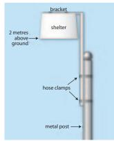
Figure 4. Installation of radiello Cartridges in Shelter
