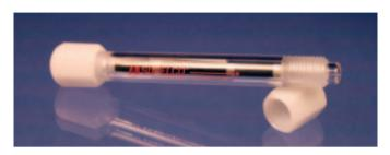
The clear body of the TDS<sup>3</sup> container is shorter than the actual tube (as shown), so the septa seals on the end of the thermal desorption tube, creating an air-tight seal.
