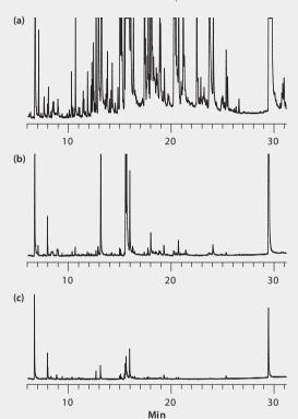
Figure 2. TICs of GC-MS/SIM Analysis of Pesticides at 50 ng/g in Beef Kidney Extract, Cleaned Using (a) Z-Sep+ and (b) PSA/C18.
