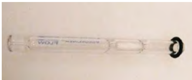
Figure 4. GC Inlet Liner after Ruggedness Testing with Olive Oil Extract Prepared using Supelclean EZ-POP NP
