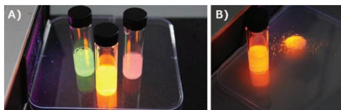
**Figure 2.** Multicolor fluorescent silica nanobeads dispersed in water and lyophilized form. Emission wavelength of the nanobeads can be tuned from blue to red and infrared.
