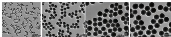
**Figure 1.** Monodispersed fluorescent silica nanobeads of different sizes. From left to right: 25 nm (Prod. No. **797901**), 50 nm (Prod. No. **797952**), 90 nm (Prod. No. **797944**), and 120 nm (Prod. No. **797871**).
