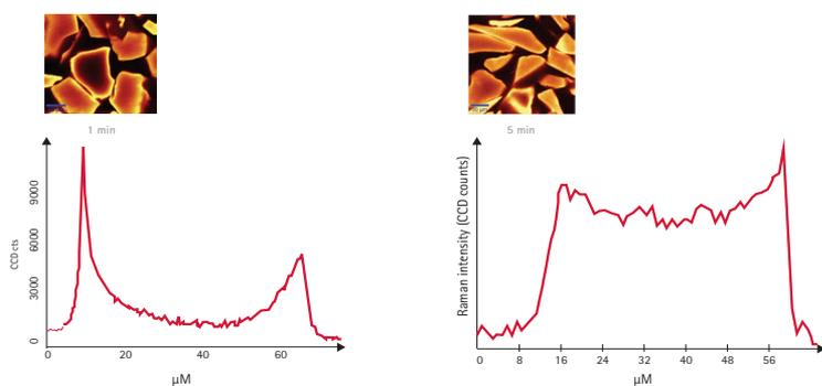
**Figure 1.** Confocal Raman microscopy of ProSep® Ultra Plus media. The bright areas on the micrographs show where the IgG has penetrated the ProSep® media. The line scans of the fluorescence intensity correlate to the IgG concentration.
