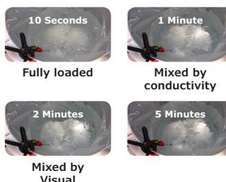
**Figure 2.** At 45 seconds, process data for mixing 1X DPBS in Mobius® Power MIX 100 shows conductivity reaching maximum value at both top and bottom of vessel. Particle count reaches minimum value at approximately 2 minutes. At same time, visual mixing is complete as the liquid becomes clear. No further changes in visual were seen after 2 minutes, confirming complete mix at that time.
