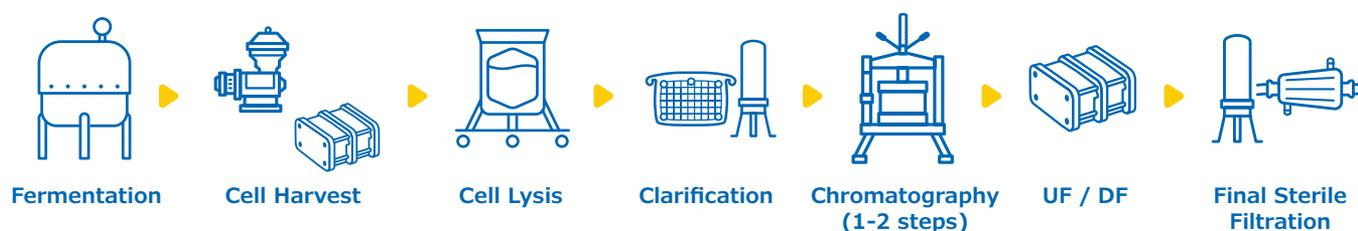
**Figure 1:** General process flow for pDNA manufacturing
