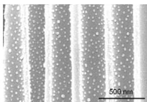
**Figure 4.** Cross-sectional SEM images of a porous alumina membrane coated with a PAA/PAH/Au nanoparticle film. The gold nanoparticles were stabilized by citrate. Used by permission of the American Chemical Society.<sup>14</sup>
