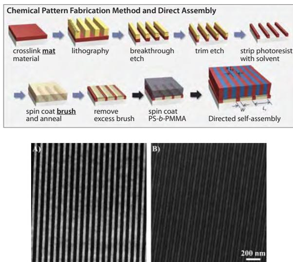
**Figure 4.** Schematic of the chemical pattern fabrication process for density multiplication using lamellae forming PS-*b*-PMMA. (Reprinted with permission from ACS.<sup>29</sup>) **A)** SEM image of the patterned photoresist (period = 80 nm), **B)** SEM image of the block-copolymer film (period = 40 nm) on top of the pattern in **A**.
