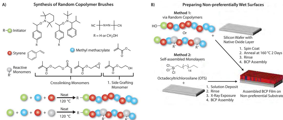
**Figure 1.** Synthesis of random copolymers (A) and the two methods of preparation of non-preferential surfaces (B). Non-preferential surfaces are formed by either spin coating and annealing random copolymers (Method 1), or forming a self-assembled monolayer and exposing to x-rays (Method 2). After preparation of the non-preferential surface, a block copolymer (BCP) can be spin coated onto the surface, and then annealed to achieve its equilibrium morphology.
