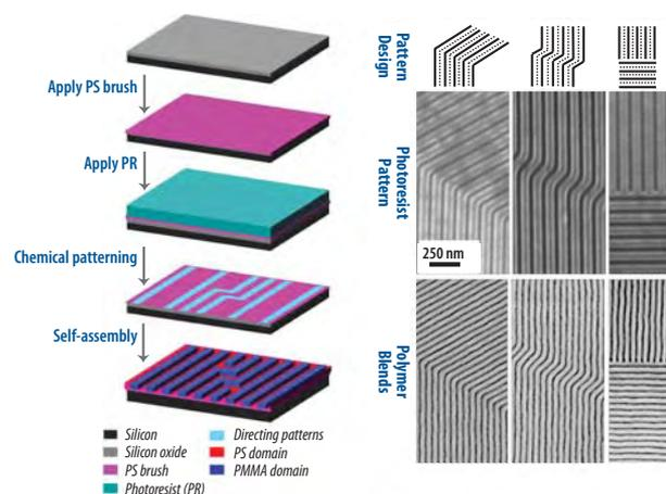
**Figure 5.** On the left is shown a schematic of the directed assembly process for the directed assembly of a block copolymer into device-oriented geometries with density multiplication. On the right is shown the chemical pattern design (top row), SEM images of the photoresist pattern (middle row), and the corresponding block copolymer-homopolymer ternary blends (bottom row) directed to assemble into device-oriented structures.<sup>35</sup>
