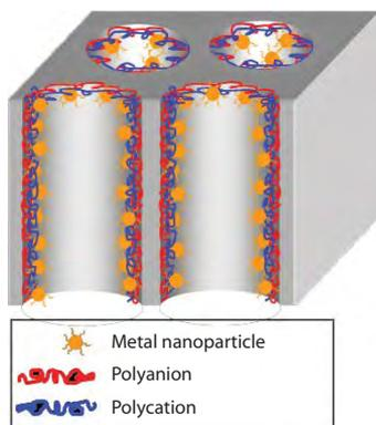
**Figure 3.** Schematic drawing of catalytic metal nanoparticles immobilized in a porous membrane using LbL deposition. Used by permission of the American Chemical Society.<sup>14</sup>
