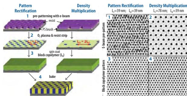
**Figure 3.** On the left is shown a schematic of the chemical pattern fabrication process for the directed assembly of cylinder-forming PS-*b*-PMMA, for both with (right) and without (left) density multiplication. 1-2) SEM images of the patterned photoresist. 3-4) SEM images of the block copolymer film on top of prepatter defined by the corresponding pattern above.<sup>28</sup>
