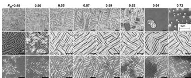
**Figure 2.** Effect of mole fraction of styrene ( $F_{St}$ ) in a P(S-*r*-MMA) brush on the orientation of self-assembled films of PS-*b*-PMMA. The rows of top-down SEM images correspond to lamellae forming (top), PMMA cylinder forming (middle), and PS cylinder forming (bottom) PS-*b*-PMMA. Black scale bars correspond to 200 nm. Reprinted with permission from ACS.<sup>26</sup>
