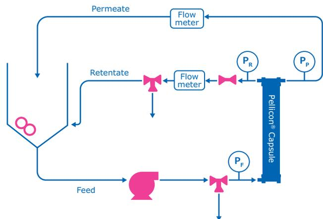
**Figure 1.** Schematic of TFF system setup.
