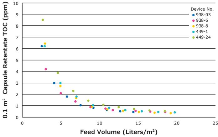
**Figure 1.** Evaluation of retentate TOC by feed volume for capsule size 0.1 m<sup>2</sup>.
