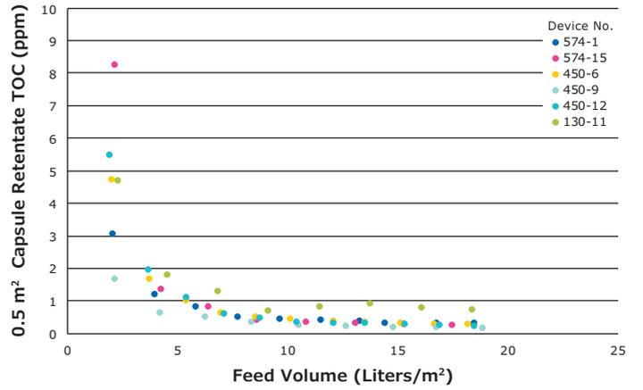
**Figure 2.** Evaluation of retentate TOC by feed volume for capsule size 0.5 m<sup>2</sup>.
