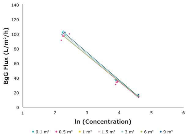
**Figure 3.** Flux vs ln BgG concentration trendline fit for mass transfer (slope) calculation of capsules.
