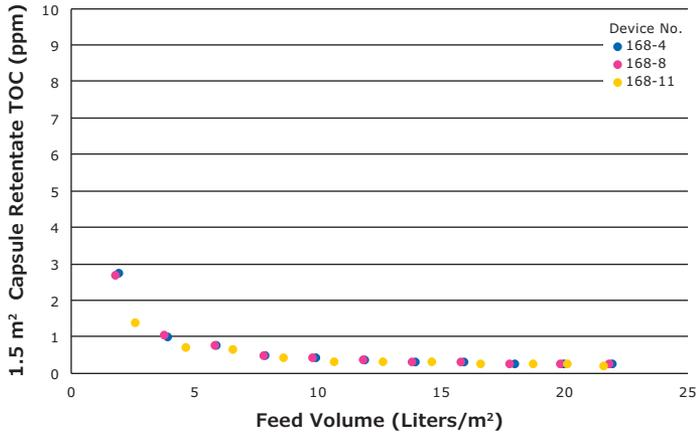
**Figure 3.** Evaluation of retentate TOC by feed volume for capsule size 1.5 m<sup>2</sup>.
