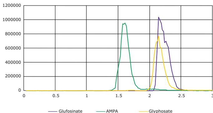
**Figure 3.** LC/MS Analysis of Glyphosate, AMPA, and Glufosinate using Supel™ Carbon HPLC column. Quantitative transitions are shown for each analyte. Conditions are described in the experimental section. 100 ng/mL calibration standard is shown.
