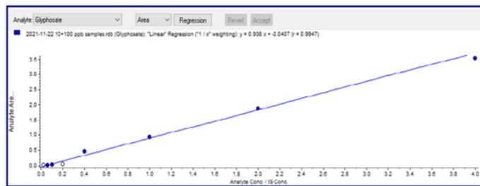
**Figure 4.** Representative calibration curve for glyphosate
