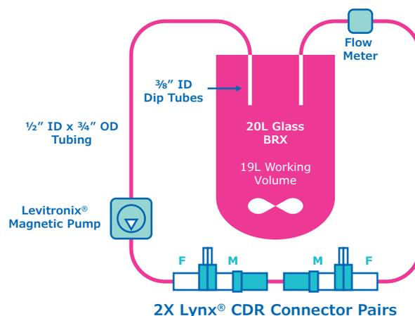
**Figure 4.** Schematic depiction of the cell shear loop assembly employed for Study A. A tubing loop containing 2 Lynx® CDR Connector pairs was aseptically connected to a 20 L glass bioreactor. A Levitronix® pump was used to circulate a cell-containing fluid stream through the experimental system at 16.5 LPM.
