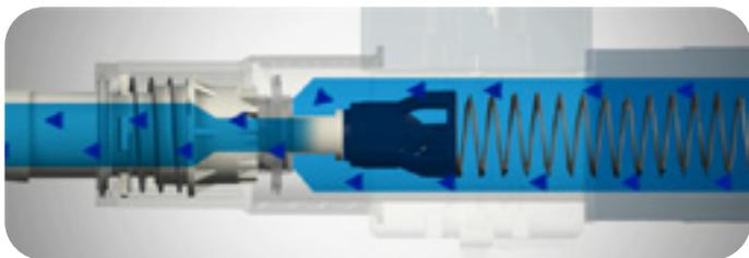
**Figure 3.** The Lynx® CDR Connector flow path diagram. Note that the diagram depicts fluid flow from right to left. Fluid movement occurs around internal components within the actuated device; it is not strictly a straight through path.
