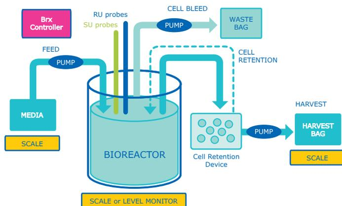
**Figure 2.** Schematic depiction of a perfusion set up in bioreactors. The bioreactor is fed with fresh media at the same rate at which spent media is removed. A cell retention device is used to separate spent media from cells in the bioreactor generating the recombinant product. In some applications, cell bleeds are periodically conducted to maintain operational control within the bioreactor.
