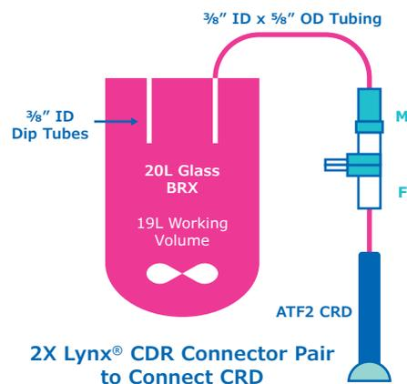
**Figure 5.** Schematic depiction of the XCell™ ATF 2 System-based perfusion operation utilizing a Lynx® CDR Connector pair employed for Study B. The XCell™ ATF 2 System was sterilely connected to a 20 L glass bioreactor using the Lynx® CDR Connector, flexible tubing, and a submerged dip tube installed in the head plate of the bioreactor.
