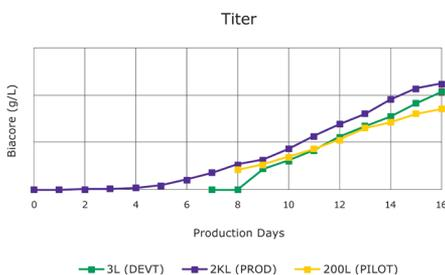
**Figure 7.** Comparison of titers for the three bioreactor sizes
