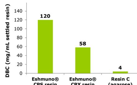
Figure 1: Dynamic binding capacities of cation exchange resins at 10 % breakthrough for rh growth factor at 36 mS/cm.
