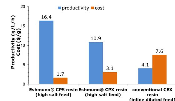
Figure 4: Costs and productivities associated with application of different types of cation exchange resins in rh growth factor purification.
