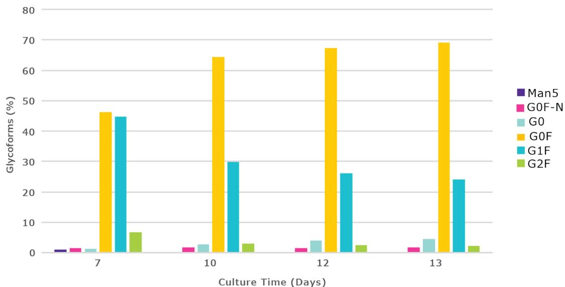
**Figure 5:** N-glycosylation profile during the 13 Day fed-batch process for CHOZN® mAb2 cultured in a Mobius® 50L single-use bioreactor using EX-CELL® Advanced CHO fed-batch medium fed 50:50 EX-CELL® Advanced CHO Feed 1 and Cellvento® 4Feed.
