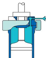
Pneumatically assisted axial displacement technology ensures fast, efficient, and homogeneous bed packing.
