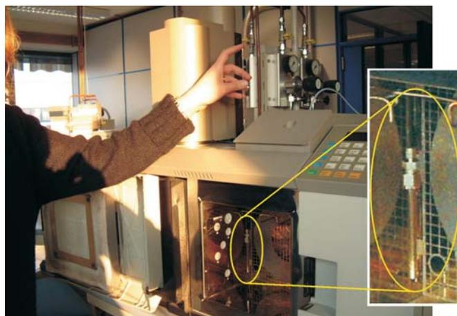
*Calibration standards are easy to prepare by applying to the gas chromatograph injector a Swagelok reducing connection (1/16 to 1/4"); injections are performed through a GC injector, where a short piece of wide-bore (0.53 mm i.d.) deactivated uncoated column is installed.*
