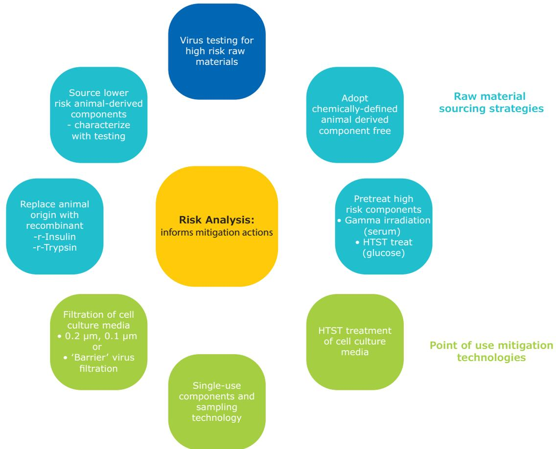
**Figure 8.** Different options to mitigate upstream viral contamination.
