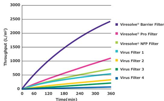
Figure 6. Comparison of traditional downstream virus filters (1-4), the Viresolve® NFP and Viresolve® Pro downstream virus filters and the Viresolve® Barrier filter designed specifically for processing cell culture media.
