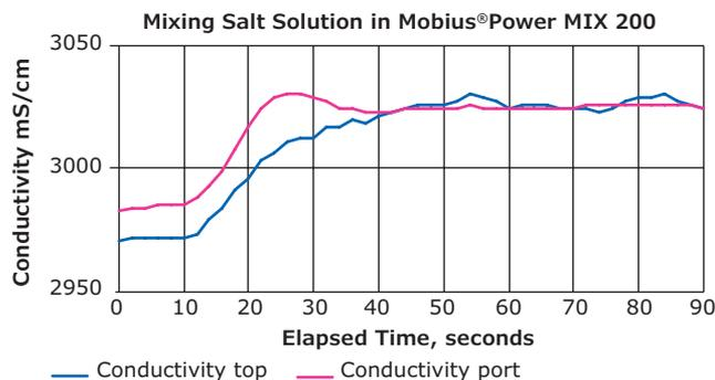
**Figure 7.** Example of conductivity trace for full speed and full volume, where mixing is complete in 25 seconds, as measured by reaching t99 (99% of final value).
