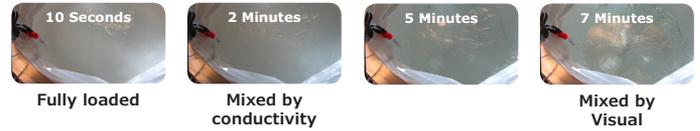
**Figure 3.** At 2 minutes, conductivity readings at both the top and bottom of the vessel reach a stable value, indicating homogeneity in mixing 1.5M NaCl in the Mobius® Power MIX 200. The solution begins to become clear at 5 minutes, with complete clarity to the bottom of the vessel at 7 minutes. At 9 minutes, particle count reaches a minimum, stable reading.
