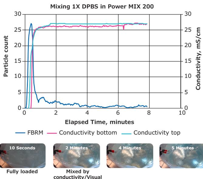
**Figure 2.** At 90 seconds, process data for mixing 1X DPBS in Mobius® Power MIX 200 shows conductivity reaching final value at both top and bottom of vessel. Visual mixing is complete as the liquid becomes clear between 2 and 4 minutes. Particle count reaches minimum value at approximately 4 minutes. No further changes in visual were seen after 4 minutes, confirming complete mix at that time.
