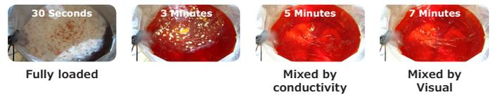
**Figure 4.** At 5 minutes, process data for mixing DMEM in Mobius® Power MIX 200 shows conductivity reaching final value. At this time, only a few small agglomerates of powder are visible. These last pieces are slowly dissolving. At 7 minutes, visual mixing is complete with no visible powder on the surface or in the liquid. The solution appears very clear. Particle count reaches a minimum between 6-9 minutes.
