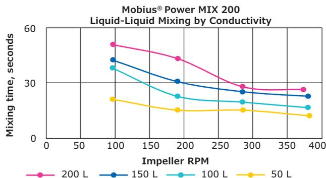
**Figure 8.** Mixing Characterization Map for Mobius® Power MIX 200
