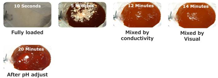
**Figure 5.** While mixing Ex-Cell® Advanced™ medium in Mobius® Power MIX 200, conductivity reaches a stable value at 12 minutes. The last of the powder is incorporated at 14 minutes for complete visual mixing. Particle count reaches maximum at 14 to 16 minutes. After pH adjustment, particle count goes to minimum, with an associated increase in conductivity. Q.S. to 200L decreases conductivity.
