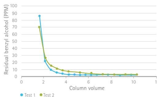
**Figure 2.** Benzyl alcohol clearance data for ProSep® Ultra Plus media
