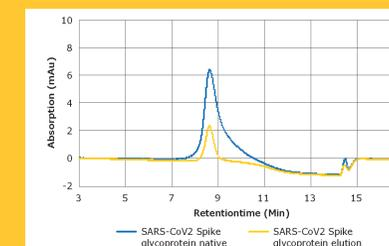
**Figure 8** - Analytical results of the sample fraction characterization using a HIC analytical method displayed in UV traces of analyzed elution fraction, including loaded glycoprotein (load) at 1 mg glycoprotein/mL CV loading.
