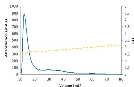
**Figure 5** - Example of pH (yellow) and UV (blue) traces detected for the chromatographic flow-through separation of oligo-mannose containing monoclonal antibody sample loaded to 10 mg/mL CV on the mixed mode cation exchange resin.
