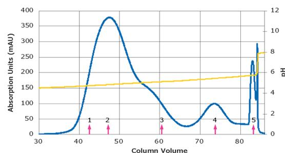
**Figure 3** - Example of pH (yellow) and UV (blue) traces detected for the chromatographic separation of an oligo-mannose containing monoclonal antibody sample loaded to 20 mg/mL CV on the mixed mode cation exchange resin. Pink marking indicates the fractions collected during the sample elution. 150 cm/h velocity was chosen throughout all the chromatographic steps.
