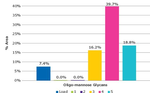
**Figure 4** - Analytical results of the sample fraction characterization using a LC-MS analytical method displayed in quantitative area of analyzed elution fractions (1 to 5), including loaded glycoprotein (load) at 20 mg glycoprotein/mL CV loading.
