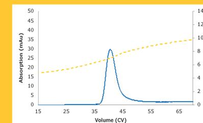
**Figure 7** - Example of pH (yellow) and UV (blue) traces detected for the chromatographic separation of oligo-mannose glycan containing protein (e.g., SARS-CoV2 Spike glycoprotein) sample loaded to 1 mg/mL CV on the mixed mode cation exchange resin.
