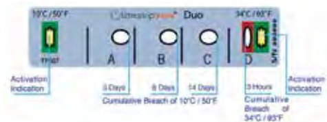
Figure 2 Timestrip Duo 10 °C and 34 °C is a customized version of two temperature breach indicators in one label.
