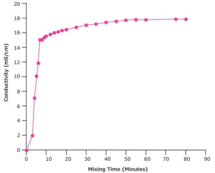
**Figure 5.** Conductivity vs. Mixing Time Using a Peristaltic Pump for Mixing.
