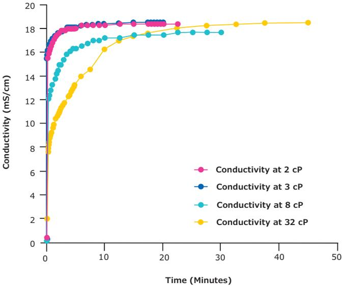
**Figure 3.** Conductivity vs. Mixing Time at 2 cP, 3 cP, 8 cP, and 32 cP at 23°C.
