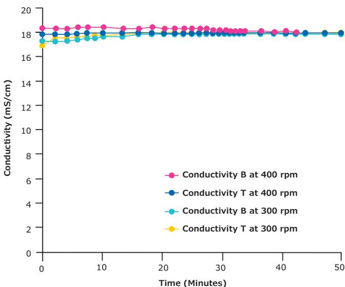
**Figure 1.** Conductivity vs. Mixing Time at 300 rpm and 400 rpm.
