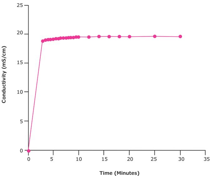
**Figure 4.** Conductivity vs. Mixing Time While Operating in a Cold Room.
