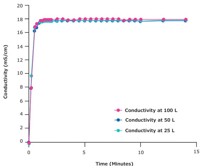
**Figure 2.** Conductivity vs. Mixing Time at 100 L, 50 L, and 25 L at 400 rpm.
