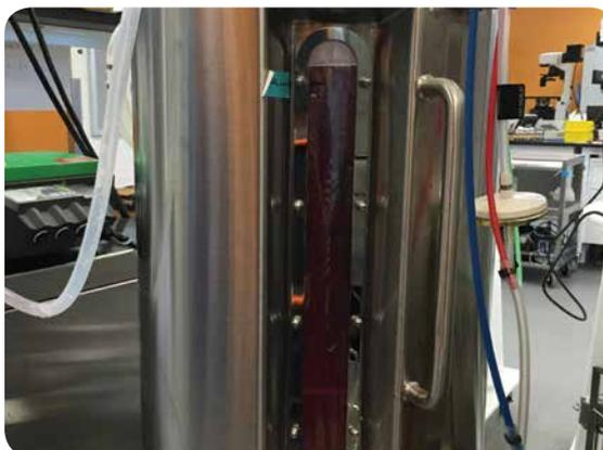
**Figure 8.** Mobius® Bioreactor on day 14 of the cell culture process simulation. The media is clear, indicating no contamination.
