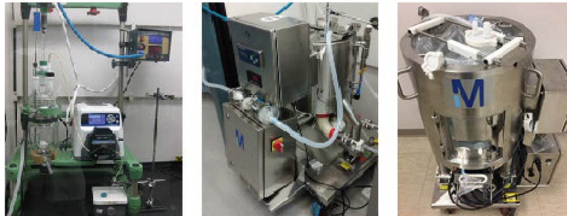
Figure 1: Conjugation vessels used in demonstration batch (left, glass vessel), pilot batch (middle, single-use vessel) and GMP batch (right, single-use vessel)
