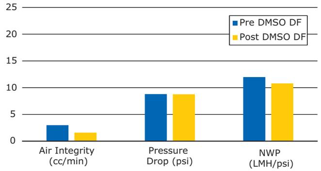
**Figure 4.** Air integrity, pressure drop, and NWP evaluation before and after DMSO diafiltration.
