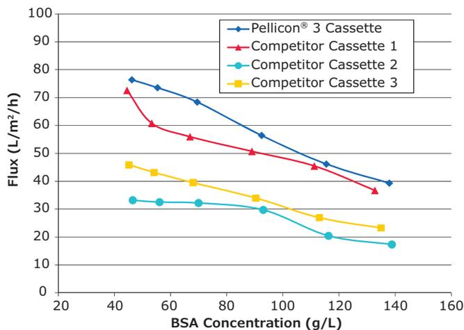
Figure 4. Comparison of Protein Flux vs Protein Concentration at 5 LMM of tested cassettes.
