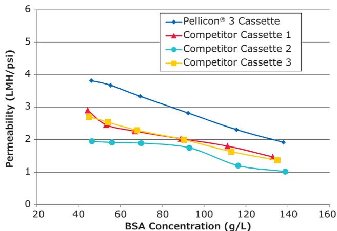
Figure 5. Comparison of Protein Permeability vs BSA Concentration at 5 LMM of tested cassettes.
