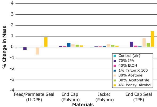
**Figure 1.** Change in mass of tested materials of construction after chemical soaks.
