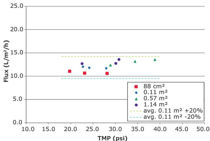
**Figure 4.** Permeate Flux vs TMP of Pellicon<sup>®</sup> 3 cassettes with 30 kDa Ultracel<sup>®</sup> membrane and D screen processing a 200 g/L HgG solution.
