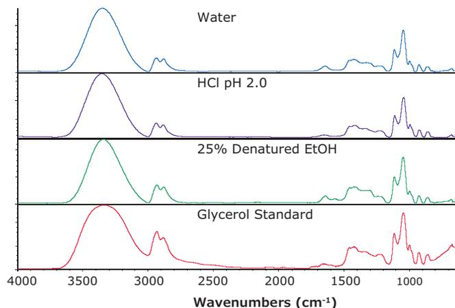
**Figure 1.** FTIR spectra of extracts from Pellicon® 3 cassettes show the presence of glycerol.
