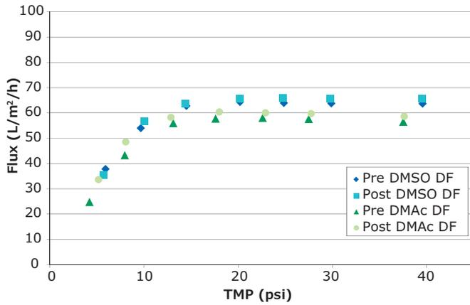
**Figure 2.** Flux vs TMP of Pellicon® 3 cassettes with 30 kDa Ultracel® membrane at 20 g/L BgG solution before and after DMSO and DMAc diafiltration.
