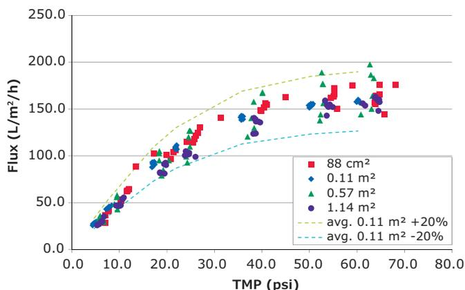
**Figure 2.** Permeate Flux vs TMP of Pellicon<sup>®</sup> 3 cassettes with 10 kDa Ultracel<sup>®</sup> membrane and C screen processing a 20 g/L BSA solution.
