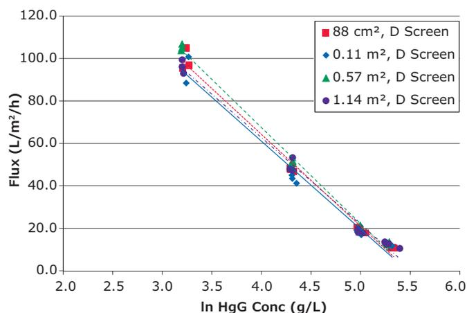
**Figure 5.** Flux vs ln HgG Concentration at 6 L/min/m<sup>2</sup> trendline fit for mass transfer calculation (slope) of Pellicon® 3 cassettes with Ultracel® membrane and D screen.
