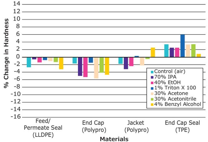
**Figure 2.** Change in hardness of tested materials of construction after chemical soaks.
