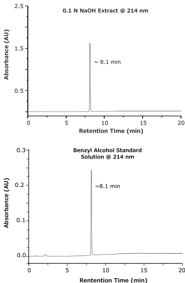
**Figure 2.** RP-HPLC chromatograms of the 0.1 N NaOH extract solution (top) and benzyl alcohol standard solution (bottom).
