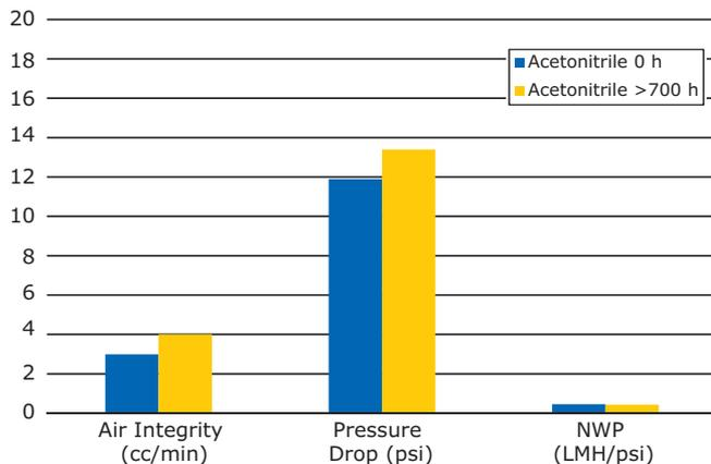
**Figure 2.** Air integrity, pressure drop, and NWP evaluation before and after acetonitrile exposure.
