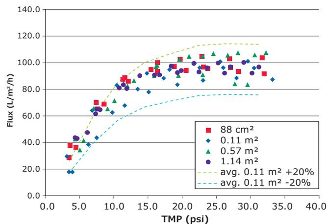
**Figure 3.** Permeate Flux vs TMP of Pellicon<sup>®</sup> 3 cassettes with 30 kDa Ultracel<sup>®</sup> membrane and D screen processing a 25 g/L HgG solution.
