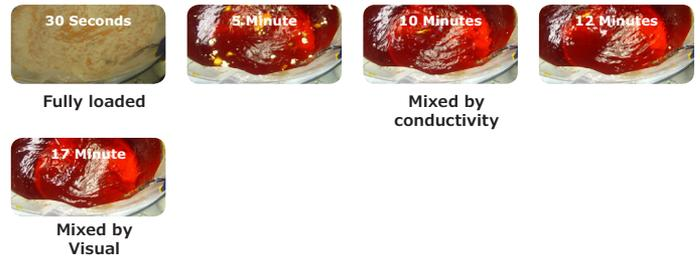
**Figure 4.** At 10 minutes, process data for mixing DMEM in Mobius® Power MIX 500 shows conductivity reaching final value. At this time, only a few small agglomerates of powder are visible. These last pieces are slowly dissolving. At 17 minutes, visual mixing is complete with no visible powder on the surface or in the liquid. Particle count appears to reach a minimum between 12 to 15 minutes. At 25 minutes, with Q.S. to 500L, there is a decrease in conductivity.
