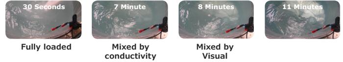
**Figure 3.** At 7 minutes, conductivity readings at both the top and bottom of the vessel reach a stable value, indicating homogeneity in mixing 1.5M NaCl in the Mobius® Power Mix 500. At this time, the solution is starting to become clear, with the impeller somewhat visible. Clarity improves greatly at 8 minutes and even more at 11 minutes, where visual mixing is deemed complete. Particle count also reaches a minimum at 9 minutes.
