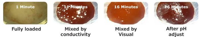
**Figure 5.** Ex-Cell® Advanced™ medium powder mixes similarly to DMEM powder. Conductivity reaches a stable value at 11 minutes. The last of the powder is incorporated at 16 minutes for complete visual mixing. Particle count appears to level out around 20 minutes, but does still increase some after that, most likely related to bubbles. After pH adjustment, particle count goes to minimum, but there is some foaming and so particle count does not reach zero.
