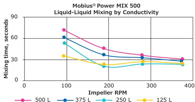
**Figure 8.** Mixing Characterization Map for Mobius® Power MIX 500
