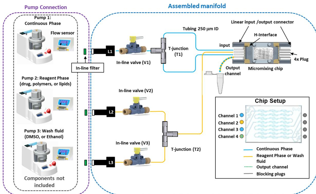
**Figure 1:** Schematic of the microfluidics setup for the Dolomite Microfluidics system. The manifold is supplied preassembled. The microfluidics chip is packaged separately. In-line filters are supplied for connection to microfluidic pumps.
