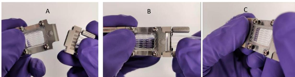
**Figure 4:** (A) Align input line from linear input/output connector and H-interface with chip, (not shown) connect output connector with blocking plugs to the other side of the H-interface (B) hand tighten the two screws on each side of the input and output connectors, and (C) check correct alignment between chip and linear input/output connector gasket
