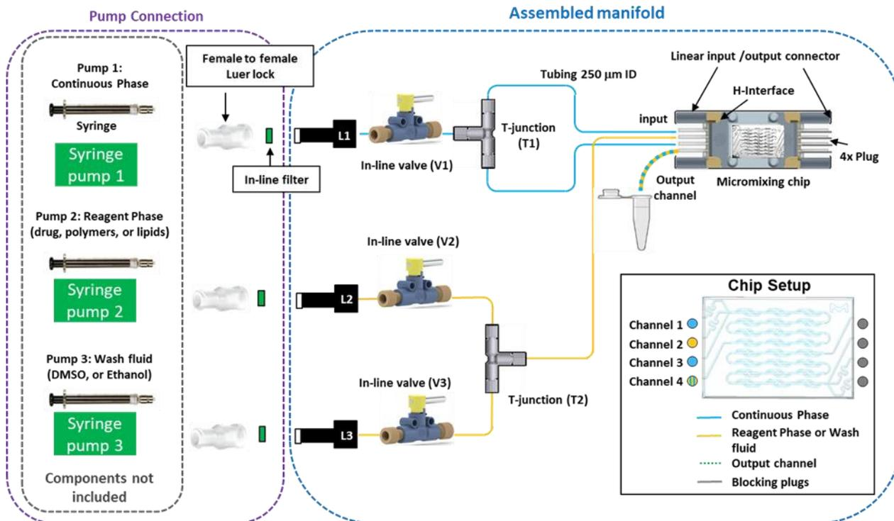
**Figure 2:** Schematic of the microfluidics setup for syringe pumps. The manifold is supplied preassembled. The microfluidics chip is packaged separately. In-line filters and luer locks are supplied for connection to syringe pumps.
