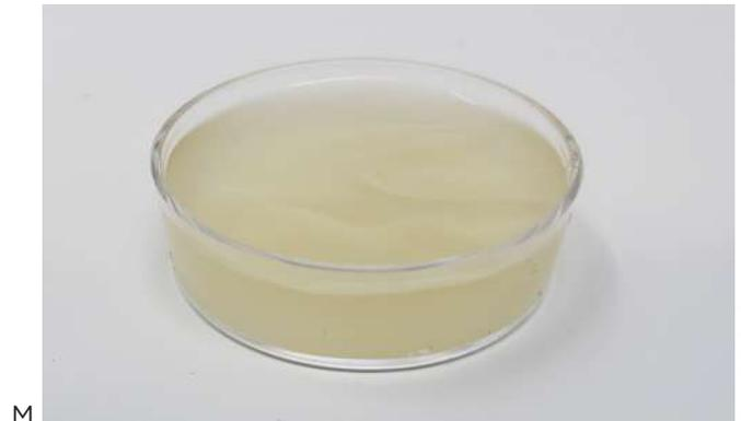
13. The bath should be as bubble-free as possible (N). Tapping firmly against the table can force large bubbles to the surface. The bath should not move easily if the container is tilted (O). Be gentle when tapping glass dishes.
