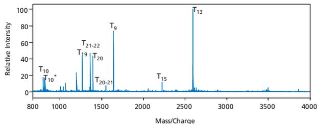
**Figure 3.** The sample was desalted using a ZipTip™ C18 pipette tip from Millipore and eluted directly onto the MALDI target using the MALDI matrix ( $\alpha$ -cyano-4-hydroxycinnamic acid, 10 mg/ml in 70% ACN, 0.03% TFA). MALDI analysis was performed in the reflection positive ion mode.
