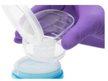
Effortless funnel separation: a simple pinch and the funnel is removed from the membrane: no forceful cracking of the plastic. The funnel lid closes the media plate which is then ready for incubation.
