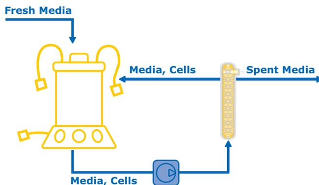
**Figure 1:** Cellicon™ filter connected to 3 L Mobius® bioreactor.
