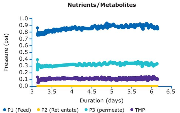
**Figure 7:** Cellicon™ filter performance during N-1 perfusion process.
