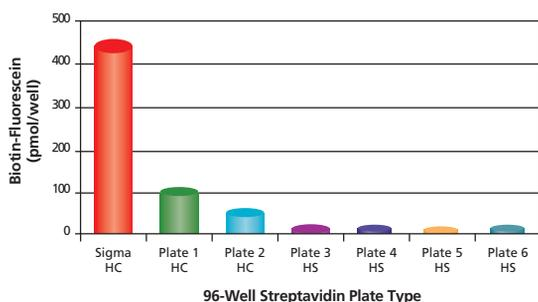
**Figure 1. Binding capacity based on biotin-fluorescein.** SigmaScreen Streptavidin HC coated plate binding capacity comparison with commercially available HC and high sensitivity (HS) streptavidin-coated plates.
