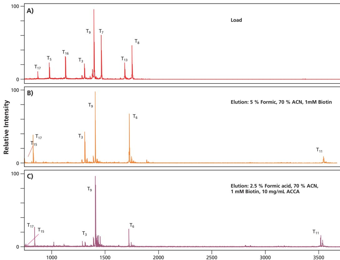
**Figure 3. MALDI-MS spectra plate load and recovery.** Spectrum (A) shows MALDI-MS analysis of trypsin-digested biotinylated lysozyme prior to loading on Streptavidin HC coated plates. Spectra (B) and (C) show purified biotinylated peptides eluted from the plates with various reagents.
