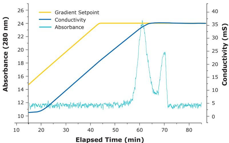
**Figure 1.** Separation of ovalbumin from trypsin inhibitor was scouted on a Vantage™ L column (22 mm). The process was then linearly scaled up (418X by volume, 20X by diameter) to a 450 mm QuikScale® column with highly comparable results.
