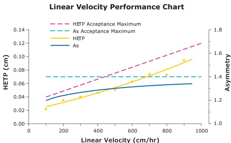
**Figure 2.** HETP/Linear Velocity/As curve for a 450 mm QuikScale® column packed with ProSep® media.
