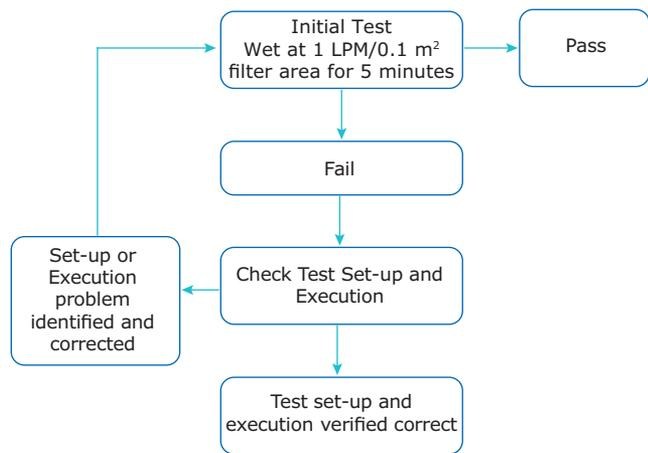
When the test is verified to be run correctly, the cause of failure must be due to one of the non-highlighted items in **Table 2**.
