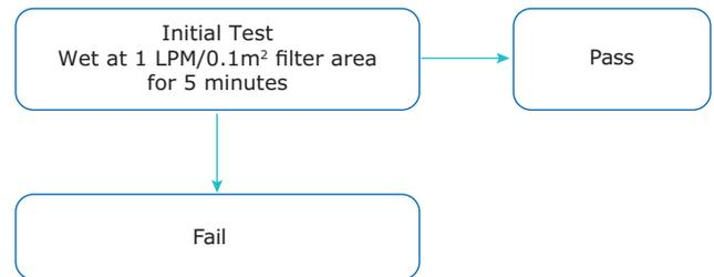
If the integrity test fails after the initial wetting procedure, often the typical reaction is simply re-wet and re-test. If the reason for initial test failure is poor wetting, simply re-wetting may fix the problem and result in a passing result. But, as we saw in Table 1, poor wetting is only one of many reasons for test failure. Ignoring the possibilities beyond poor wetting can result in repeated failures, frustration, lost time or lost product.
