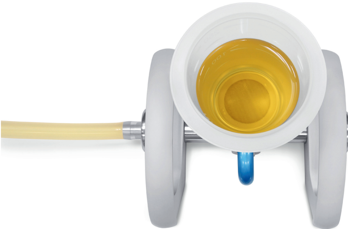
Figure 2. EZ-Fit® 1-place manifold with PVDF membrane filter and Vegetable Peptone Broth.
