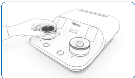
Figure 27: membrane support removal by twisting it
