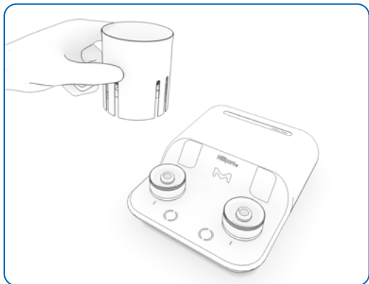
Figure 29: membrane support removal with removal tool—part 2
