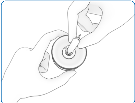
Figure 41: check valve installation with tool—part 2
