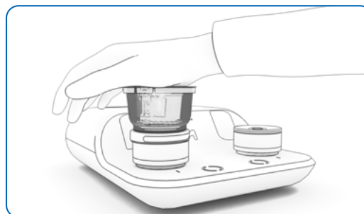
Figure 18: filtration unit lid firmly pressed down with the palm to lock
