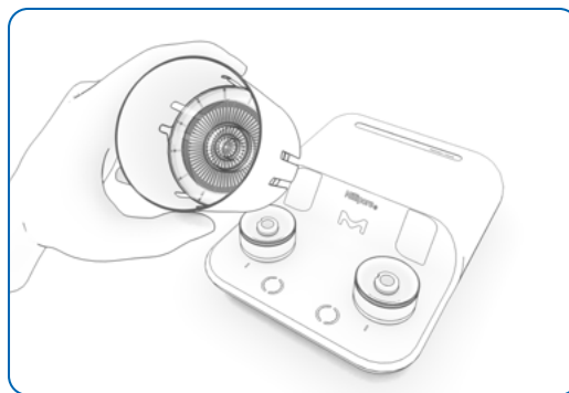
Figure 30: membrane support removal with removal tool—part 3
