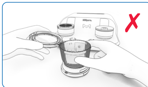
Figure 23: INCORRECT filtration unit lid removal
