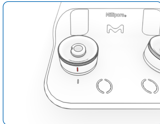
Figure 13: the sign on a locked head is aligned with the one on the pump body
