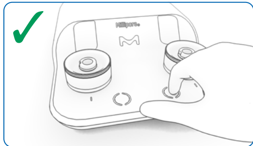
Figure 5: CORRECT finger position to start or stop the pump
