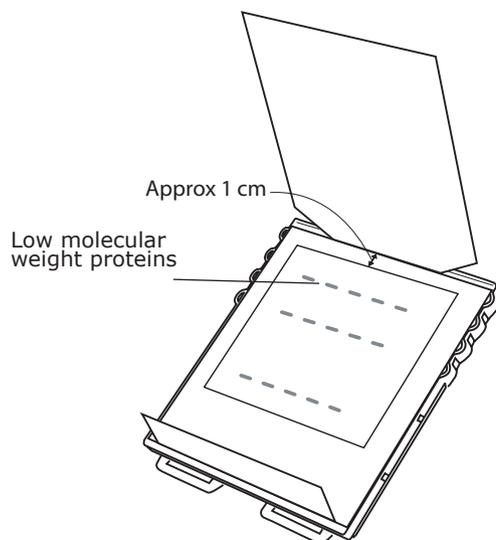
**Figure 5. Blot placement**
