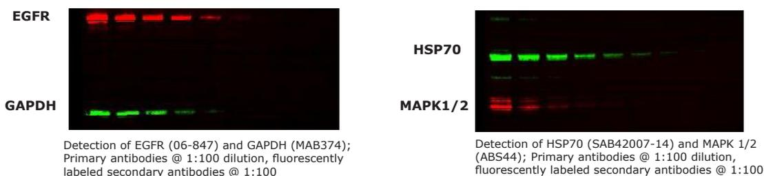
**Figure 10. Multiplex fluorescent detection with the Immobilon® GO Device**
