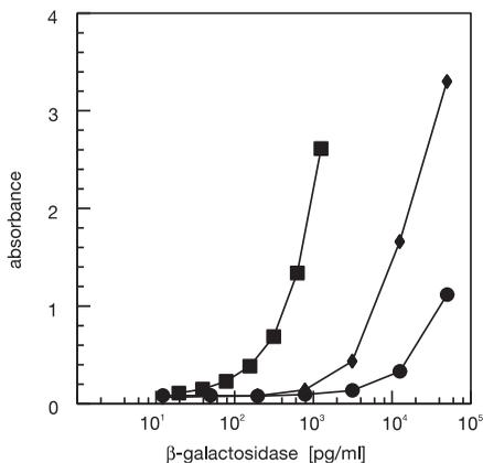
**Fig. 3: Comparison of the detection limits of colorimetric assays for  $\beta$ -galactosidase.** Colorimetric detection of  $\beta$ -galactosidase activity using ONPG (●) and CPRG (◆) as substrates is performed according to standard protocols. The  $\beta$ -Gal ELISA (■) was performed as described, using ABTS and substrate enhancer. The ELISA method is more than 10-fold more sensitivity as compared to the standard assays
