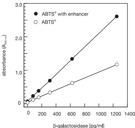
**Fig. 4:** A typical calibration curve using ABTS (20 min POD reaction) without (○) or with (●) substrate enhancer.
