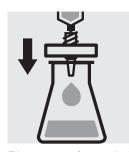
Filter or centrifuge turbid samples.
