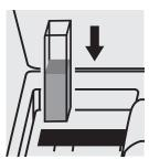
Place the cell into the cell compartment.
