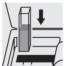
Place the cell into the cell compartment.
