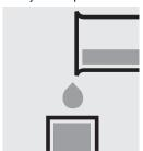
Transfer the solution into a cell.
