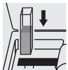
Place the cell into the cell compartment.
