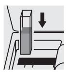
Place the cell into the cell compartment.
