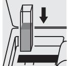
Place the cell into the cell compartment.
