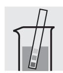
Check the pH of the sample, specified range: pH 0 - 13.
