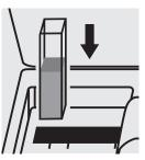
Place the cell into the cell compartment.
