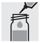
Add 1.0 ml of OA-3K with pipette, close the cell with the screw cap, and mix.
