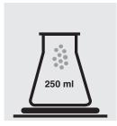
Weigh 50.0 ± 0.1 g of homogenized sample into a 250-ml conical flask.
