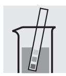
Check the pH of the sample, specified range: pH 4-9. If required, add dilute sodium hydroxide solution or sulfuric acid drop by drop to adjust the pH.
