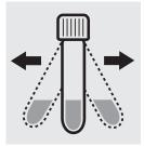
Shake both cells vigorously to dissolve the solid substance.
