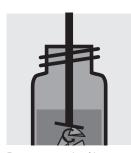
Disintegrate the filter in the homogenizer.
