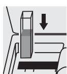
Place the cell into the cell compartment.
