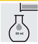
Transfer to a 50-ml volumetric flask using sulfuric acid 0.05 mol/l.
