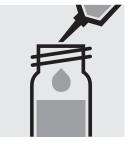
Add 5.0 ml of the sample with pipette, close the cell with the screw cap, and mix.
