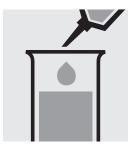
Add 0.20 ml of reagent 2 with pipette and mix.
