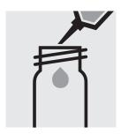
Pipette 4.0 ml of NO₃-1 into a dry empty round cell (Empty cells, Cat. No. 1.14724).
