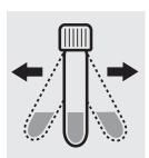
Shake the cell vigorously for 1 minute to dissolve the solid substance.
