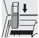
Place the cell into the cell compartment.
