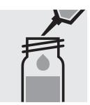
Pipette 1.0 ml of the sample into a reaction cell, close with the screw screw cap, and mix. cap, and mix.
