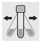
Close cell tightly and shake **vigorously** until the reagent is completely dissolved.
