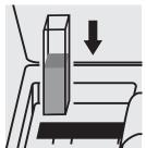
Place the cell into the cell compartment.
