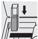
Place the cell into the cell compartment.
