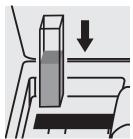
Place the cell into the cell compartment.
