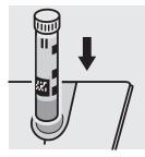
Place the **cell**  $\Sigma$  **P** into the cell compartment. Align the mark on the cell with that on the photometer.
