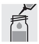
Add 1.0 ml of **H-1K** with pipette, close the cell with the screw cap, and mix.
