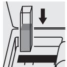
Place the cell into the cell compartment.
