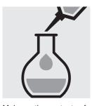
Make up the contents of the volumetric flask to the mark with isooctane for spectroscopy Uvasol® (Cat. No. 1.04718) and mix.
