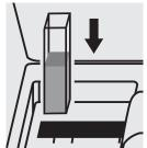
Place the cell into the cell compartment.
