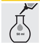
Place 1 ml of pretreated sample into a 50-ml volumetric flask.
