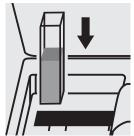
Place the cell into the cell compartment.
