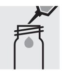
Pipette 5.0 ml of the sample into an empty round cell (Empty cells, Cat.No. 1.14724).
