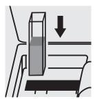
Place the cell into the cell compartment.
