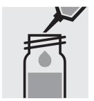
Add 1.0 ml of **reagent 1** with pipette, close the cell with the screw cap, and mix.
