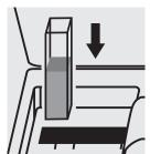
Place the cell into the cell compartment.
