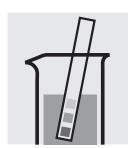
Check the pH of the sample, specified range: pH 1.5 - 2.2. If required, add dilute sodium hydroxide solution or hydrochloric acid drop by drop to adjust the pH.
