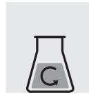
Sufficiently homogenize 0.5 - 2 I of sample. **Note** the sample volume.
