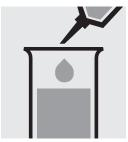
Pipette 0.05 ml of sample into a plastic vessel.
