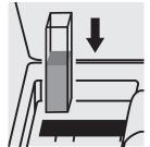
Place the cell into the cell compartment.
