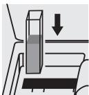
Place the cell into the cell compartment.
