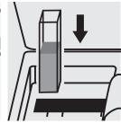
Place the cell into the cell compartment. The blank measurement is performed automatically.
