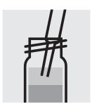
Aspirate the clear upper phase from the tube with pipette.
