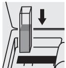
Place the cell into the cell compartment.
