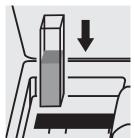
Place the cell into the cell compartment.
