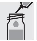
Carefully pipette 5.0 ml of the depleted blank tightly with the screw cap, cell, close tightly with the screw cap, and mix vigorously.
