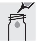
Pipette 5.0 ml of the 1:4 dilute sample into an empty round cell (Empty cells, Cat.No. 1.14724).
