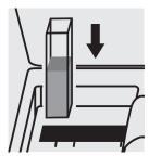
Place the cell into the cell compartment.
