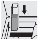
Place the cell into the cell compartment.
