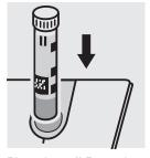
Place the **cell B** into the cell compartment. Align the mark on the cell with that on the photometer. The measurement is performed automatically.
