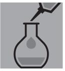
Make the contents of the volumetric flask up to the mark with ethanol, keeping them protected from light in the process!
