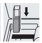
Place the cell into the cell compartment.
