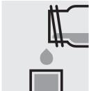
Transfer the solution into a cell.
