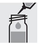
Add 0.10 ml of the sample with pipette, close the 5 minutes, measure cell with the screw cap, and mix. Caution, cell becomes hot!
