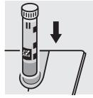
Place the **cell A** into the cell compartment. Align the mark on the cell with that on the photometer. The measurement is performed automatically.
