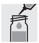
Pipette 0.50 ml of the sample into a reaction cell close with the screw cap, and mix.
