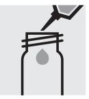
Pipette 5.0 ml of the pretreated sample into an empty round cell (Empty cells, Cat.No. 1.14724).
