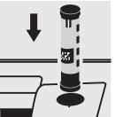
Select method with AutoSelector measuring range 5 – 150 mg/l NH<sub>4</sub>-N.
