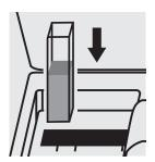
Place the cell into the cell compartment.
