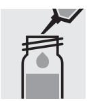
Pipette 0.50 ml of CI-1K into a reaction cell, close with the screw cap, and mix.
