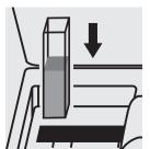
Place the cell into the cell compartment.
