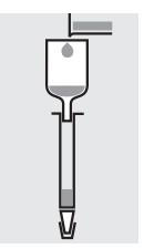
Fill 100 ml of the sample and 6 drops of **AOX-4** into the reservoir.
