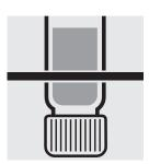
Remove the cell from the thermoreactor and let it, **standing on its head**, to cool for 1 hour.
