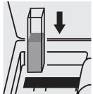
Place the cell into the cell compartment.
