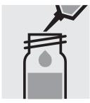
Add 2 ml of **color reagent**, close the test tube with the screw cap, and mix.
