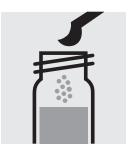
Add 1 level green microspoon of **HCHO-1K** into a reaction cell, close with the screw cap.
