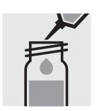
Add 5.0 ml of **Zn-6** (Cat.No. 1.06146, Isobutyl methyl ketone) with pipette and close the test tube with the screw cap.
