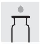
Fill 2 oxygen reaction bottles each with inoculated nutrient-salt solution and 2 glass beads to overflowing. Close bubble-free with the slanted ground-glass stoppers.
