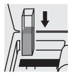
Place the cell into the cell compartment.
