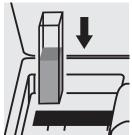
Place the blank cell into the cell compartment.
