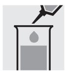
Pipette 0.25 ml of distilled water (Water for analysis EMSURE®, Cat. No. 1.16754, is recommended) or buffer solution into a plastic vessel.
