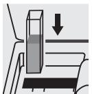
Place the cell into the cell compartment.
