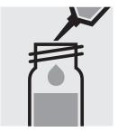
Add 5.0 ml of the pretreated sample with pipette, close with the screw cap, and mix.
