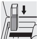
Place the cell into the cell compartment.
