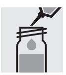
Add 5.0 ml of  $NO_3$ -2 with pipette into the cell. Close the cell with the screw cap.
