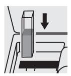
Place the cell into the cell compartment.
