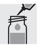
Pipette 4.0 ml of the sample into a reaction cell, close with the screw cell with the screw cap, cap, and mix.
