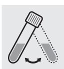
Suspend the bottom sediment in two cells by swirling.
