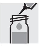
Pipette 1.0 ml of the **pretreated sample** into a reaction cell, **do not** mix!
