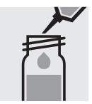
Add 8.0 ml of the sample with pipette and close with the screw cap.
