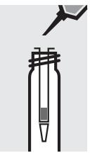
Run 3 separate 1-ml portions of **AOX-3** through the column. Discard the wash solution
