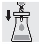
Filter sample solution through a membrane filter with 0.45  $\mu$ m pore size.
