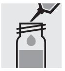
Add 1.0 ml phosphoric acid 85 % GR (Cat.No. 1.00573) with pipette, close the cell with the screw cap, and mix.
