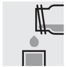
Transfer the solution into a 50-mm cell.
