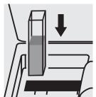
Place the cell into the cell compartment.
