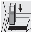
Place the cell into the cell compartment.
