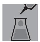
Acidify a portion of the extract with hydrochloric acid 1 mol/l Titripur® (Cat. No. 1.09057) (50 µl per 5 ml of extract).
