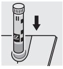
Place the **cell A** into the cell compartment. Align the mark on the cell with that on the photometer. The measurement is performed automatically.
