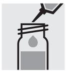
Add 2.0 ml of the sample-reagent mixture with pipette, close the cell with the screw cap, and mix.
