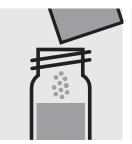
Add 1 powder pack of Molybdenum HR2, close with the screw cap, and dissolve the solid substance.
