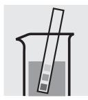
Check the pH of the sample, specified range: pH 2–10. If required, add dilute sodium hydroxide solution or sulfuric acid drop by drop to adjust the pH.
