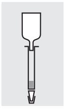
Attach the glass reservoir to the prepared column (closed at the bottom end).
