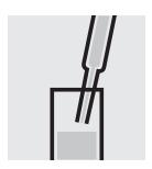
Transfer the solution into Select method no. **130**. a cell.
