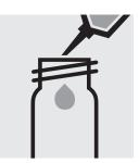
Pipette 10 ml of the sam- Add 1 drop of Cr-1K, ple into an empty round cell (Empty cells, Cat.No. and mix. 1.14724).
