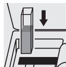
Place the cell into the cell compartment.
