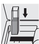
Place the cell into the cell compartment.
