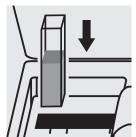
Place the cell into the cell compartment.
