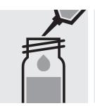
Add 0.50 ml of the sample with pipette, close the cell with the screw cap, and mix.
