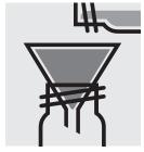
Filter the content of the test tube with a round filter into another test tube with screw cap.
