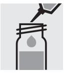
Add 5.0 ml of sulfuric acid 40 %, close the cell a corresponding cell. with the screw cap, and mix.
