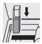
Place the cell into the cell compartment.
