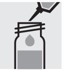
Add to each vessel 0.10 ml of **Si-2** with pipette, close with the screw cap, and mix.
