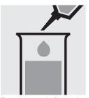
Pipette 1.0 ml of sample into a plastic vessel.
