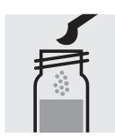
Add 1 level microspoon of **NO<sub>3</sub>-1K** into a reaction cell and close with the screw cap.
