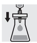
Filter or centrifuge turbid samples.
