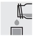
Transfer the solution into a rectangular cell.
