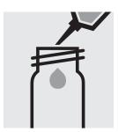
Pipette 5.0 ml of the sample into a reaction cell, close with the screw cap, and dissolve the solid substance.
