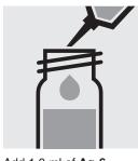
Add 1.0 ml of Ag-6, close with the screw cap, and mix.
