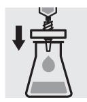
Filter sample solution through a membrane filter with 0.45  $\mu$ m pore size.
