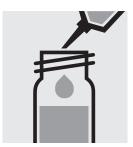
Add 10 ml of n-butyl acetate and close the test tube with the screw cap.
