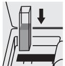
Place the cell into the cell compartment.
