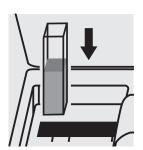
Place the cell into the cell compartment.
