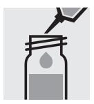
Pipette 0.10 ml of the sample into a reaction cell close with the screw cap, and mix.
