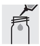
Pipette 5.0 ml of NO₃-1 into a dry empty round cell (Empty cells, Cat. No. 1.14724).
