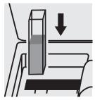
Place the cell into the cell compartment.
