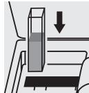
Place the cell into the cell compartment.
