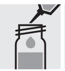
Add 1.0 ml of the sample with pipette, close the cell with the screw cap, and mix.
