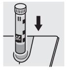
Place the blank cell into the cell compartment. Align the mark on the cell with that on the photometer.
