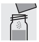
Add 1 powder pack of **Oxyscav 1** and close with the screw cap.
