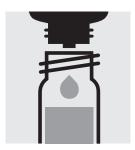
Add 3 drops of **Mg-2K**, close the cell with the screw cap and mix.
