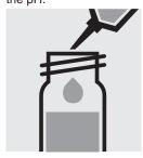
Add 7.0 ml of distilled water with pipette to the second reaction cell, close with the screw cap, and mix. (Blank)
