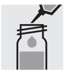
Pipette 0.20 ml of AOX-1K into a reaction cell, and mix.
