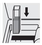
Place the cell into the cell compartment.
