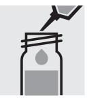
Add 10 ml of the sample with pipette, close with the screw cap, and mix.
