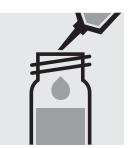
Pipette 2.0 ml of the sample into a test tube with screw cap.
