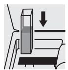
Place the cell into the cell compartment.
