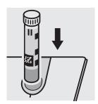
Place the cell containing the sample into the cell compartment. Align the mark on the cell with that on the photometer.
