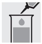
Add 2.5 ml of **Bradford** reagent solution with pipette and mix.
