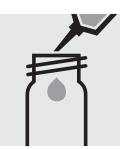
Pipette 10 ml of the sample into a plastic vessel (Flat-bottomed tubes, Cat.No. 1.17988).
