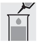
Pipette 5.0 ml of  $NH_4-1$  into a test tube.
