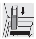
Place the cell into the cell compartment.
