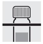
Remove the cell from the thermoreactor and place in a test-tube rack to cool to room temperature:
