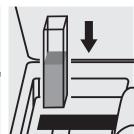
Place the cell into the cell compartment.
