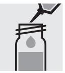
Pipette 0.100 ml of distilled water (Water for analysis EMSURE®, Cat. No. 1.16754, is recommended) into a test tube with screw cap.
