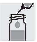
Add 1.5 ml of **B-2** with pipette and close with the screw cap.
