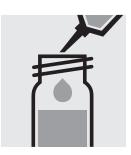
Add 6.0 ml of **B-6** with pipette, close with the screw cap, and mix.
