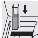
Place the **cell A** into the cell compartment.
