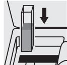
Place the blank cell into the cell compartment.
