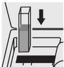
Place the cell into the cell compartment.
