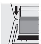
Place the cell into the cell compartment.
