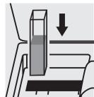
Place the cell into the cell compartment.
