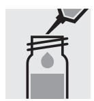
Pipette 4.0 ml of the sample into a reaction cell. Close with the screw cap.
