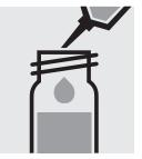
Add 0.50 ml of T-1K with Swirl the cell for pipette and close with the screw cap.
