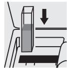
Place the cell into the cell compartment.
