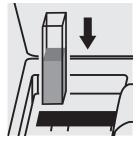
Place the cell into the cell compartment.
