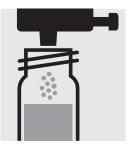
Add 1 dose of Cr-2K using the blue dosemetering cap, close the reaction cell with the screw cap.
