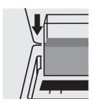
Place the cell into the cell compartment.
