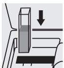
Place the cell into the cell compartment.
