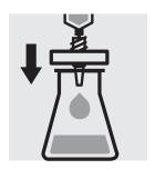
Filter or centrifuge turbid samples.
