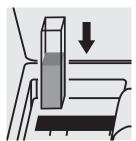
Place the cell into the cell compartment.
