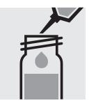
Pipette 0.20 ml of the sample into a reaction cell, close with the screw metering cap, close the cap, and mix.
