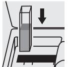
Place the cell into the cell compartment.
