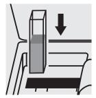
Place the cell into the cell compartment.
