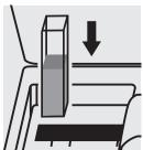
Place the cell into the cell compartment.
