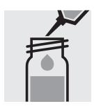
Add 2.0 ml of **DNSA** reagent with pipette, close the vessel, and mix.
