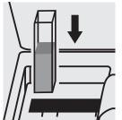
Place the cell into the cell compartment.
