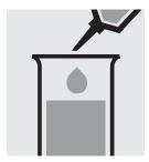
Add 2.0 ml of **Biuret** reagent solution with pipette and mix.
