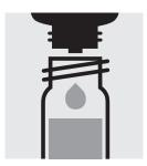
Add 3 drops of **Mn-2K**, close the cell with the screw cap, and mix.
