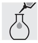
Dilute the sample with distilled water (Water for analysis EMSURE®, Cat. No. 1.16754, is recommended) in the ratio 1:200 (1+199).
