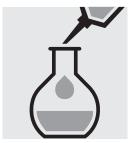
Add 20 ml of sodium molybdate/ascorbic acid reagent and mix.
