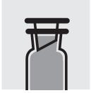
Incubate one bottle of pretreated sample and one of inoculated nutrient-salt solution closed in a thermostatic incubation cabinet at 20 ± 1°C for 5 days.
