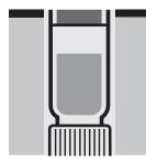
Heat the cell, standing on its head, at 120 °C in the thermoreactor for 2 hours.
