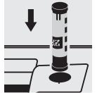
Select method with AutoSelector measuring range 2.5 – 25.0 mg/l Cl.
