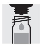
Add 2 drops of **Ni-2K**, close the cell with the screw cap, and mix.
