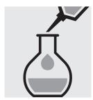
Make up the contents of the volumetric flask to the mark with sulfuric acid 0.05 mol/l and mix thoroughly: solution 1.
