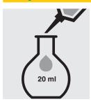
Place 10 ml of sodium molybdate/ascorbic acid reagent into a 20-ml volumetric flask.
