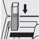
Place the cell into the cell compartment.
