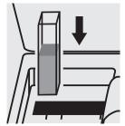
Place the cell into the cell compartment.
