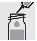
Carefully pipette 3.0 ml of the depleted blank tightly with the screw cap, cell, close tightly with the screw cap, and mix vigorously.
