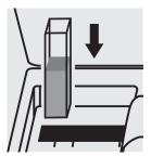
Place the cell into the cell compartment.
