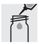
Pipette 5.0 ml of the sample into a round cell.
