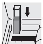
Place the cell into the cell compartment.
