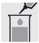
Pipette 5.0 ml of **NH<sub>4</sub>-1** into a test tube.
