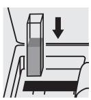
Place the **cell A** into the cell compartment.
