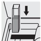
Place the cell into the cell compartment.
