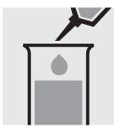
Pipette 5.0 ml of distilled Add to each tube 1.0 ml water (Water for analysis EMSURE®, Cat.No. 1.16754, is recommended) into a second test tube. (Blank)
