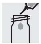
Pipette 5.0 ml of the sample into a round cell.
