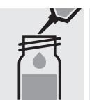
Carefully pipette 5.0 ml of the depleted sample into a reaction cell, close into a second reaction and mix vigorously. Caution, the cell becomes hot!
