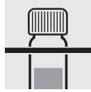
Remove the cell from the thermoreactor and place in a test-tube rack to cool to room temperature.
