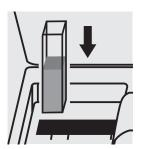
Place the cell into the cell compartment.
