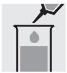
Add 0.20 ml perchloric acid 70 - 72 % GR (Cat.No. 1.00519) with pipette and mix.
