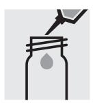
Pipette 4.0 ml of **AC-1** into a round cell.
