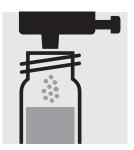
Add 1 dose of PO<sub>4</sub>-2K using the blue dosemetering cap, close the cell with the screw cap.
