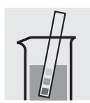
Check the pH of the sample, specified range: pH 3 - 8. If required, add dilute sodium hydroxide solution or sulfuric acid drop by drop to adjust the pH.
