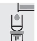
Filter the sample through a suitable filter (e.g. glass-fibre filter).
