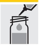
Add 2.0 ml of hydrochloric acid 6 mol/l with pipette, close the vessel, and mix.
