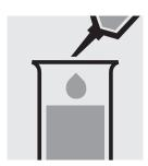
Add 0.20 ml of reagent 2 with pipette and mix.
