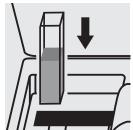
Place the cell into the cell compartment.
