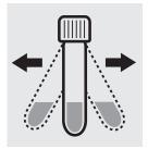
Shake the tube vigorously for 1 minute to dissolve the solid substance.
