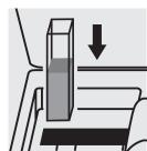
Place the cell into the cell compartment.
