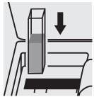
Place the cell into the cell compartment.
