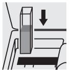
Place the cell into the cell compartment.
