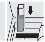
Place the cell into the cell compartment.
