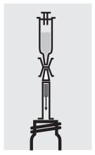
Fill the 10-ml syringe with Add 2 level green micro- Heat the cell at 120 °C 10 ml of reagent AOX-5 and attach the syringe with the column outlet using the connector. Place the top end of the column on an empty cell and rinse the charcoal filling of the column into an empty 16-mm cell.
