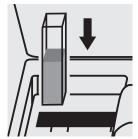
Place the cell into the cell compartment.
