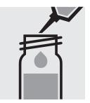
Add 1.0 ml of **H-1K** with pipette, close the cell with the screw cap, and mix.
