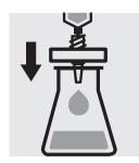
Filter sample solution through a membrane filter with 0.45 µm pore size.
