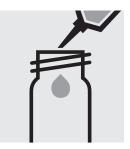
Add 10 ml of the sample into an empty round cell (Empty cells, Cat.No. 1.14724).
