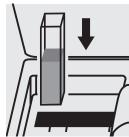
Place the cell into the cell compartment.
