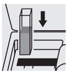
Place the cell into the cell compartment.
