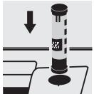
Select method with AutoSelector measuring range 2.0 – 75.0 mg/l NH<sub>4</sub>-N.
