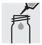
Pipette 4.0 ml of the sample into an empty round cell (Empty cells, Cat.No. 1.14724).
