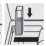
Place the cell into the cell compartment.
