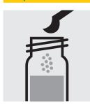
Add 1 level grey microspoon of **Pb-2K** to the already measured cell, close the cell with the screw cap.
