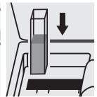
Place the cell into the cell compartment.
