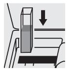
Place the cell into the cell compartment.
