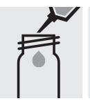
Pipette 10 ml of distilled water (Water Ultrapur, Cat.No. 1.01262, is recommended) into a second plastic vessel (Flatbottomed tubes, Cat. No. 1.17988). (Blank)
