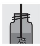
Disintegrate the filter in the homogenizer.
