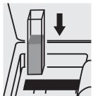
Place the cell into the cell compartment.
