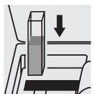
Place the cell into the cell compartment.
