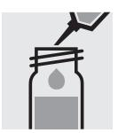
Pipette 7.0 ml of the sample into a reaction cell, close with the screw cap, and mix.
