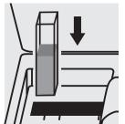
Place the cell into the cell compartment.
