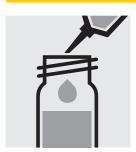
Pipette 3.0 ml of stirred sample into a reaction cell.
