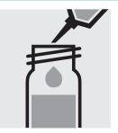
Pipette 5.0 ml of the sample into a test tube with screw cap.
