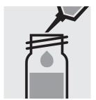
Add 10 ml of n-butyl acetate and close the test tube with the screw cap.
