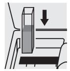
Insert the cell containing the sample into the cell compartment.
