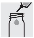
Pipette 1.0 ml of **B-1K** into a reaction cell, close with the screw cap, and mix.
