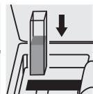
Place the cell into the cell compartment.
