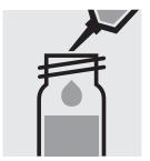
Add 0.50 ml of **Ca-2K** with pipette, close the cell with the screw cap, and mix.
