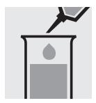
Pipette 2.0 ml of F-1 into Add 5.0 ml of water and 0.5 ml of the sample with pipette and mix.
