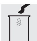
Place 1 level grey microspoon of **SO**<sub>3</sub>-1 into a dry test tube.
