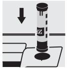
Select method with AutoSelector measuring range 1.0 – 15.0 mg/l Ca.
