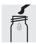
Place 1 microspoon of NO<sub>3</sub>-1 into a dry empty round cell (Empty cells, Cat.No. 1.14724).
