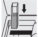
Place the cell containing the sample into the cell compartment.
