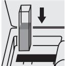
Place the cell into the cell compartment.
