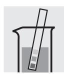
Check the pH of the sample, specified range: pH 4 – 10. If required, add dilute sodium hydroxide solution or sulfuric acid drop by drop to adjust the pH.
