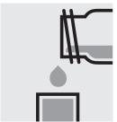
Transfer the solution into a rectangular cell.
