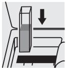
Place the cell into the cell compartment.
