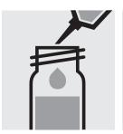
Pipette 10 ml of the sample into a reaction cell, close with the screw cap, and mix.
