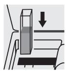
Place the cell into the cell compartment.
