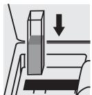
Place the cell into the cell compartment.
