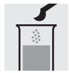
Add 1 level blue microspoon of NH<sub>4</sub>-2 (from Spectroquant® Ammonium Test, Cat. No. 1.14752).
