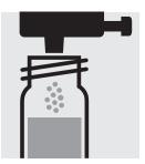
Add 1 dose of **NH**<sub>4</sub>-1**K** using the blue dosemetering cap, close the cell with the screw cap.
