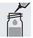
Add 0.5 ml of **Co-1K** with pipette, close with the screw cap, and mix.
