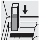
Place the cell into the cell compartment.
