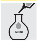
Place 20 ml of sulfuric acid 0.05 mol/l into a 50-ml volumetric flask.
