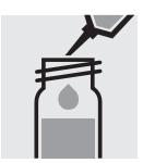
Pipette 5.0 ml of the sample into a reaction cell, close with the screw cap, and mix.
