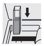
Place the cell into the cell compartment.
