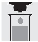
Add 2 drops of Cl<sub>2</sub>-3, close with the screw cap, and mix.
