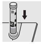
Place the **cell**  $\Sigma$  **P** into the cell compartment. Align the mark on the cell with that on the photometer.
