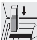
Place the cell into the cell compartment.
