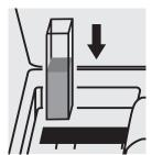
Place the cell into the cell compartment.
