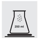
Weigh 50.0 ± 0.1 g of homogenized sample into a 250-ml conical flask.
