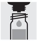
Add 2 drops of Zn-2, close the test tube with the screw cap, and mix.
