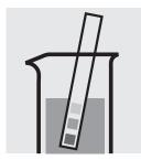
Check the pH of the sample, specified range: pH 1 – 12. If required, add dilute ammonia solution or nitric acid drop by drop to adjust the pH.
