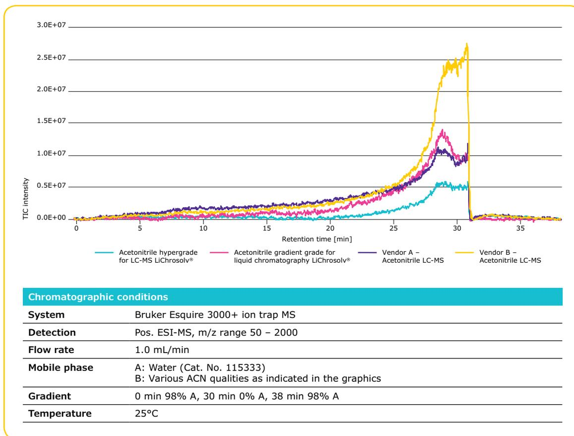
**Figure 9.** Combined TICs of the blank runs of four different acetonitrile qualities. All solvents were delivered to the MS source via an LC system.
