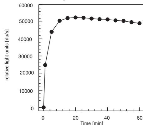
**Fig. 3:** Kinetics of light reaction. 100 pg alkaline phosphatase (intestinal) in a volume of 10 µl was detected in a black microtiter plate with 150 µl substrate reagent according to section 2.1. The light signal was measured on a Berthold LB 96 P Luminometer with 1 s integration time.
