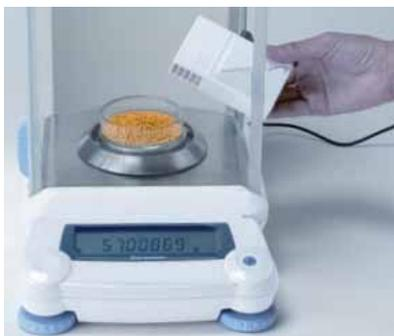
Use as hand-held device inside weighing chamber.
