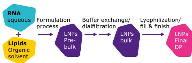
**Figure 6.** Workflow of manufacturing a lipid-based RNA formulation.
