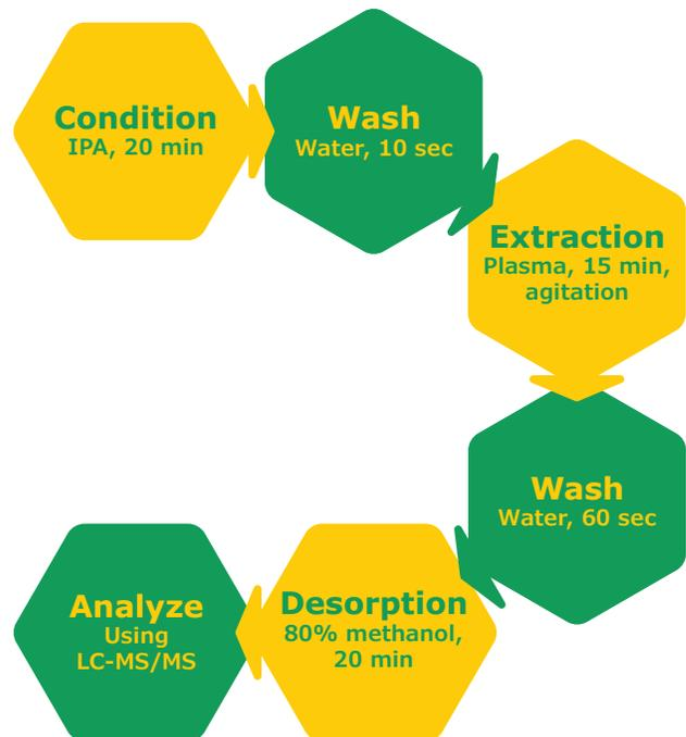
1. **Conditioning**—Program the robot to immerse the pin device into the conditioning plate (100% 2-propanol) for 20 minutes without shaking.
