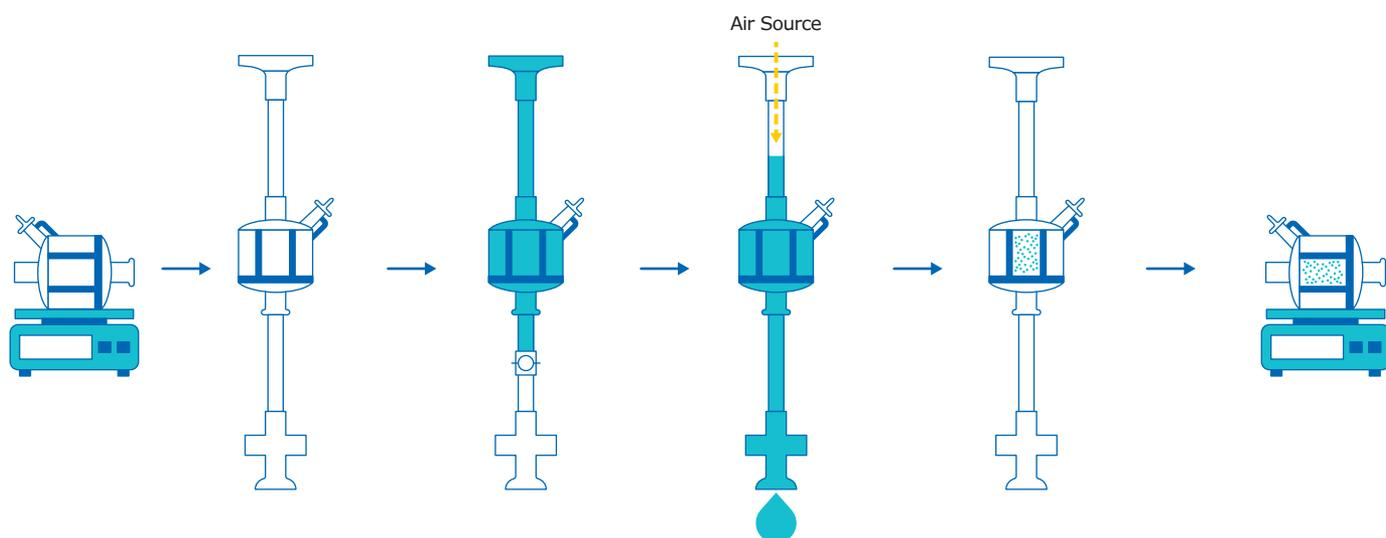
**Figure 1B.** Filter Drain by Inlet Blow-down
