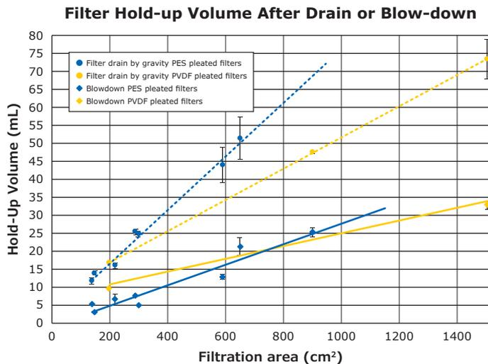
**Figure 2.** Mean hold-up volume of pleated PES (shown in blue) and PVDF (shown in yellow) filters following a filter drain (dashed lines) or a 1-minute blow-down with air at 20 psi above the filter bubble point specification (solid lines). Each value represents the mean and SD from three replicate filters.
