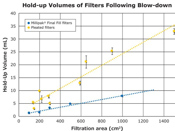
**Figure 4.** Mean hold-up volume of pleated filters compared to Millipak® Final Fill filters following a 1-minute blow-down with air at 20 psi above the filter’s bubble point specification. Each value represents the mean and SD from three replicate filters.
