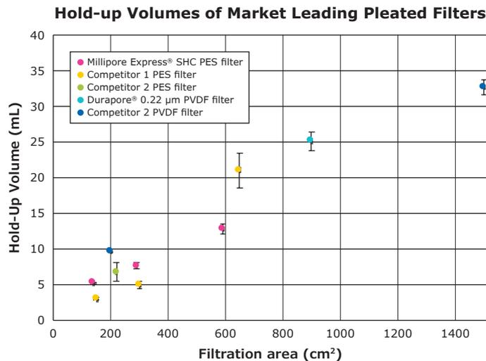
**Figure 3.** Mean hold-up volume of pleated PES and PVDF filters following a 1-minute blow-down with air at 20 psi above the filter bubble point specification. Each value represents the mean and SD from three replicate filters.
