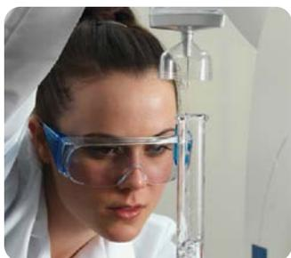
Easily prepare solutions with the low flow function to precisely adjust the meniscus in volumetric flasks.
