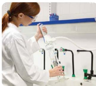
The 75 cm long tubing reaches the sink for easy glassware washing at mid or high flow (up to 2 L per min).
