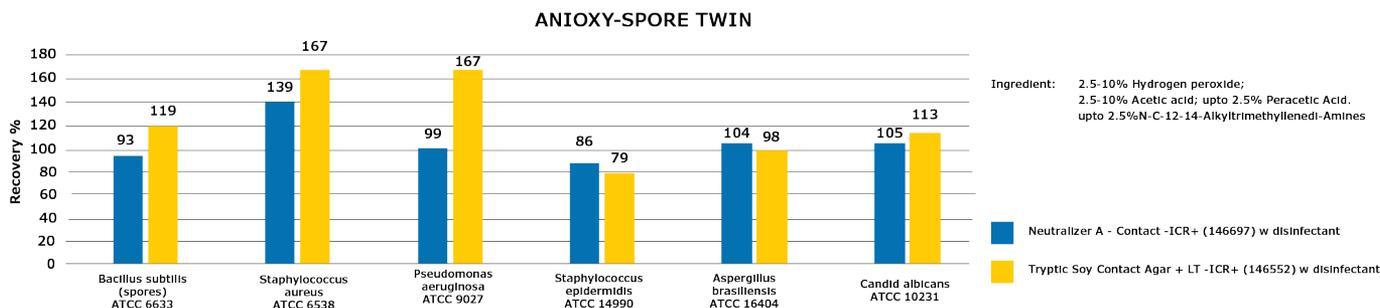
The test results show that all tested microorganism strains could be recovered in the presence of 25 µL Anioxy Spore-Twin IP sterile concentrate, indicating the efficient neutralization of active residues of this disinfectant by the contained neutralizers (**Figure 4**).
