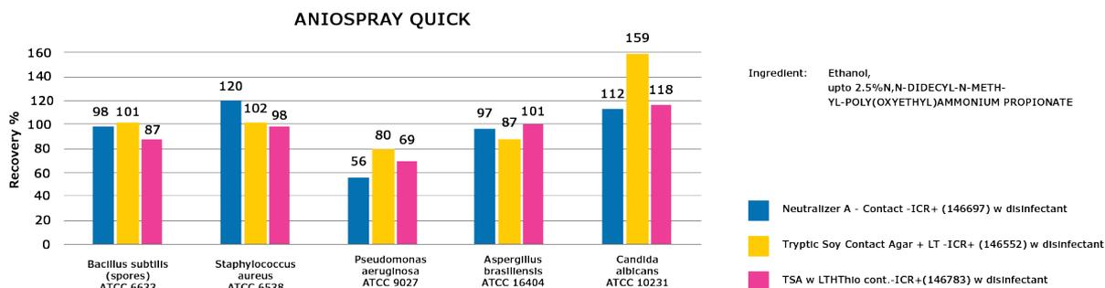
The results in **Figure 5** show that all tested microorganism strains could be recovered in the presence of 25 µL ANIOSPRAY QUICK, indicating the effective neutralization of active residues
