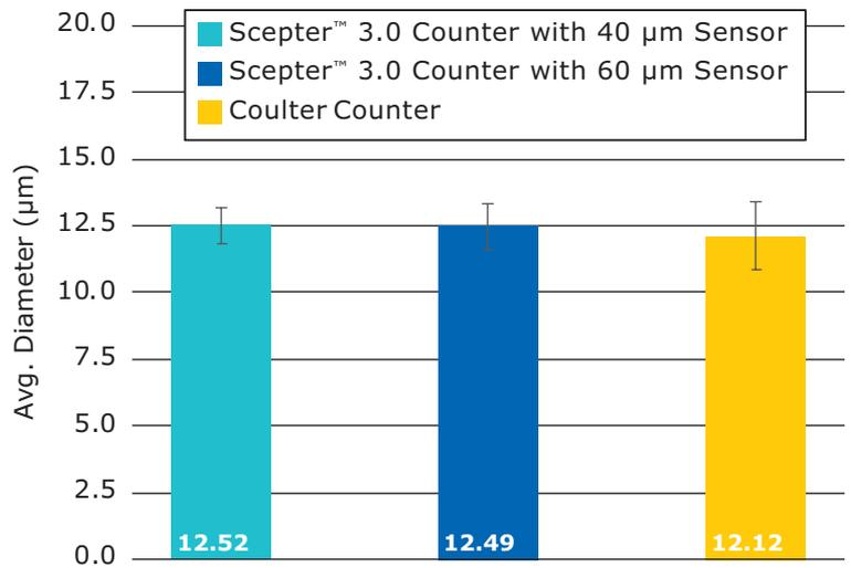
Jurkat cells were measured to test accuracy and reproducibility of cell size measurements using the Scepter™ 3.0 Cell Counter with both 40 µm and 60 µm sensors. Results are compared to the same measurement obtained with a Coulter Counter Z2™ Instrument equipped with 100 µm aperture. Data are from five measurements per sample.
