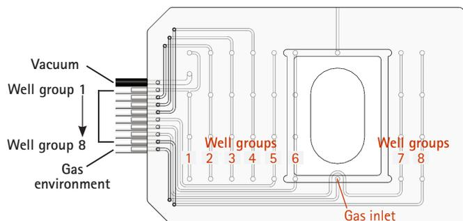
Figure 4. Lines to CellASIC® ONIX2 Microfluidic System
