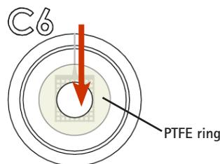
Figure 7. Well 6 cell inlet
